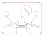
Align the windshield rubber part with the windshield holes and then install it.
