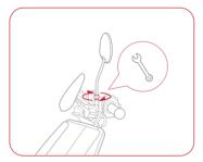
Adjust the rearview mirrors to an appropriate position and then tighten nuts on the rearview mirror with a spanner. Properly set the dust cover. Install the right rearview mirror in the same way.
