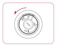
Insert the key to the main lock and turn to the icon of "OPEN" as shown in the left figure.
