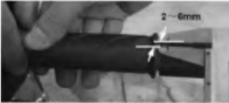
If the throttle free-play is insufficient or too large, make adjustments as necessary.
